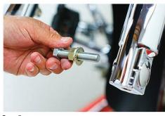
Step 5. Install the wheel with the spacers on the correct side. Apply anti-seize to the axle and thread into the captive nut first by hand.
