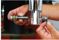
Step 1. Remove the current axle, making note of axle spacer orientation. Prepare to install captive nut (splined cap with internal threads) into the left fork leg. Thread the ½-20 nut on the bolt all the way up to its head, then the washer as pictured.
