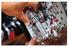
Step 9. Install right lower leg clamp using a  $\frac{1}{2}$ " socket, torque to 132-180 in-lbs.
