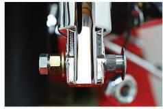
Step 2. Insert the bolt thru the axle hole from the inside of the fork leg. Thread the captive nut onto the bolt as far as you can by hand.
